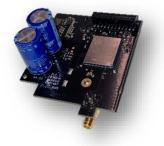
PUMA's communication module is equipped with a built-in power bank and can send voltage failure alarms if the primary power supply stops working.
