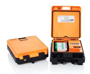
GEKKO is equipped with 2 pcs. analog inputs which are 0/4-20mA or with 4 digital inputs, 2 of which can be configured as 0-10V inputs or as pulse inputs for counter. In addition, RS485 MODBUS communication with external devices is possible..
