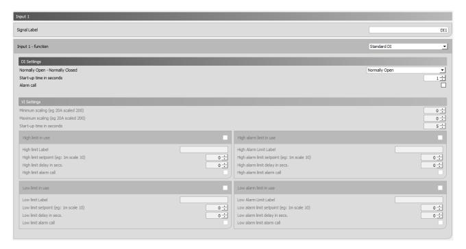
I1-2 input on the GEKKO logger can be used as either standard 0-10 V inputs, or standard DI where "0" <5V and "1"> 12V.
