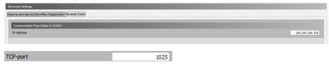
Enter the IP address and TCP port of the server on which AcowaCore is installed. The GEKKO logger will then be a TCP client and connect to the SCADA system via AcowaCore.
