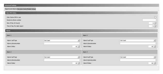
If the GEKKO is used as a stand-alone device that is not connected to a SCADA system via AcowaCore, it is possible to receive a daily status SMS and alarm SMS in case of an alarms.
