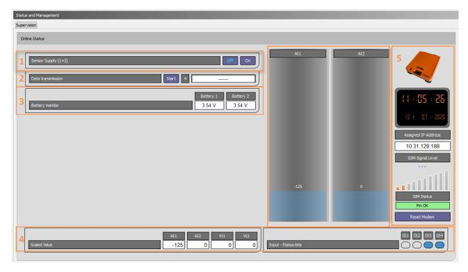
It is possible to switch the power supply for the analog inputs to on status, thereby making it possible to power and read a momentarily value from the measuring equipment which is connected (Point 4.).
