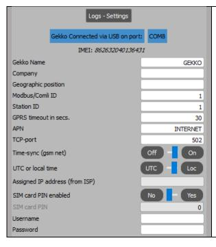
Here you will be notified if a GEKKO is connected and on which USB port it is connected.
